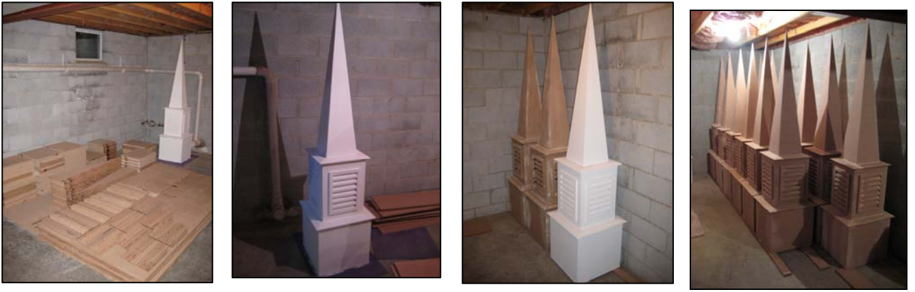
Fig 18. Cut and sized MDF wood and steeples in various stages of production. Basement Studio, Fox Run Rd, 2007
